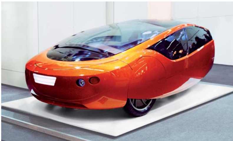
Figure 1-11: The Urbee Hybrid: the first 3-D printed car (picture courtesy of Kor Ecologic, Inc.)
